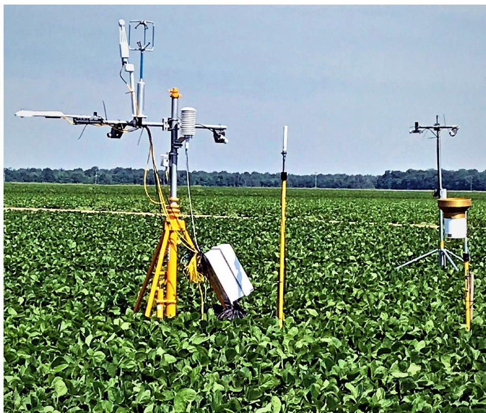
Fig. 2. The eddy covariance system installed in the soybean field for measuring evapotranspiration. The tower on the left carries the eddy covariance and energy balance monitoring systems on the same tower, and the tower on the right is for measuring spectral characteristics of soybean canopy but not used in this study.
